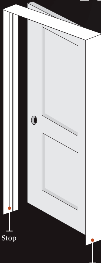
Standard Jamb Thickness \frac{3}{4} " & 1\frac{1}{16} " - we also offer custom thickness jambs.
